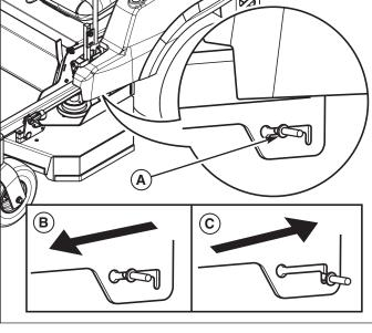
Figure 1. Transmission Release Levers (LH shown)
